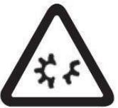
Failure to comply to this requirement may cause serious bodily harm to user or bystanders due to accidental contact with rotating impellor blades.
