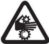
The agitator has rotating parts. Do not put your hands or fingers into a working Agitator or rotating shaft ends.
